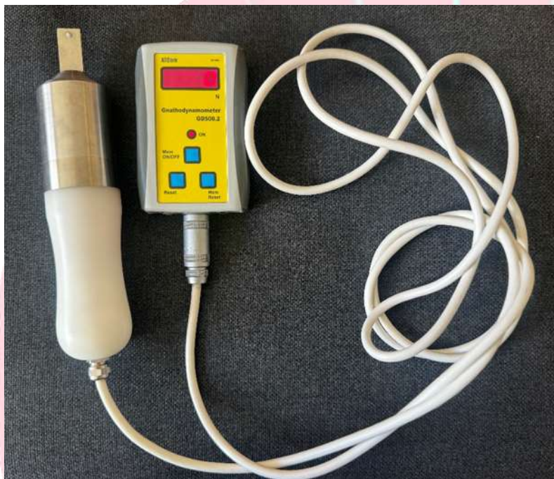
Fig.1 Gnathodynamometer - force-measuring device
