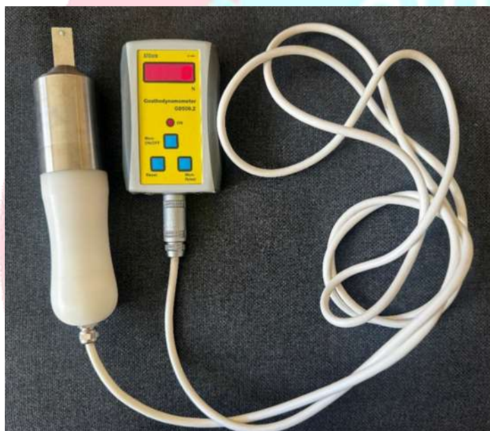
Fig.1 Gnathodynamometer - force-measuring device
